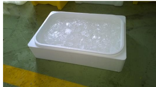
Figure 6. Ice melting experiment showing an EPS box before it was closed with a lid
